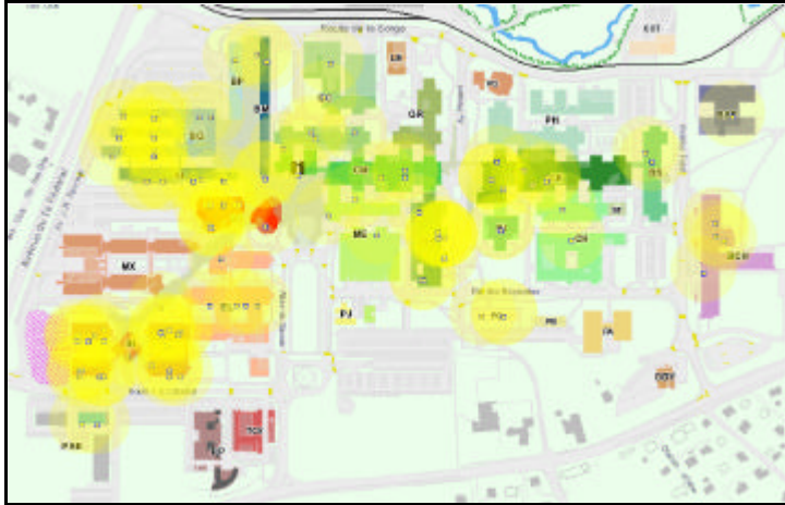
Figure 4: Wi-Fi coverage on in the campus in mid-2004. Map generated by knowing the position of the access points, not by net stumbling
