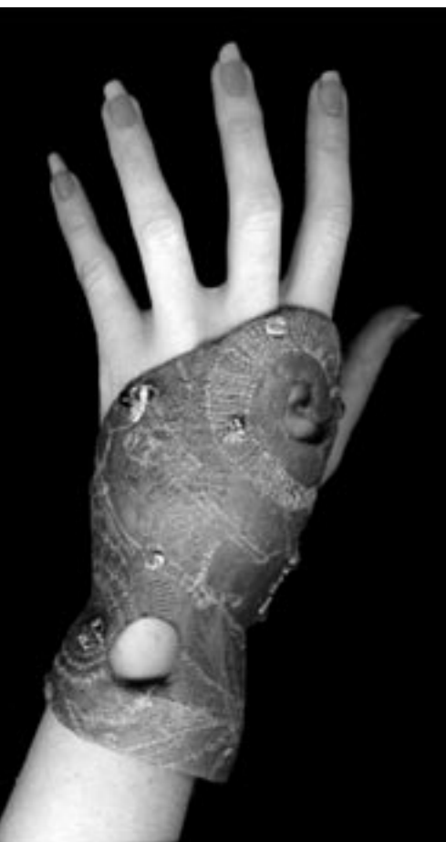
↑ Smart fashion, the armband embedded with accelerometer and bluetooth, worn to play Trickster
